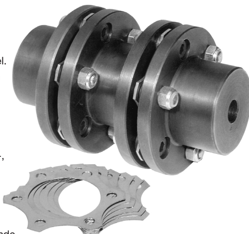
1 = Lamellpaket, 2 = Nav, 3 = Bussning, 4 = Bult, 5 = Mellandel, 6 = MIAB Fix SD 1 = Discs pack, 2 = Hub, 3 = Bushing, 4 = Screws, 5 = Spacer, 6 = MIAB FIX SD
